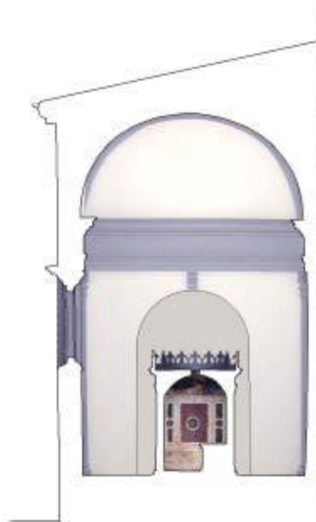
Figure 13. Cross section of the Rucellai's Chapel and the Saint Sepulcher, from the 3D model (original drawing on scale 1:50).
