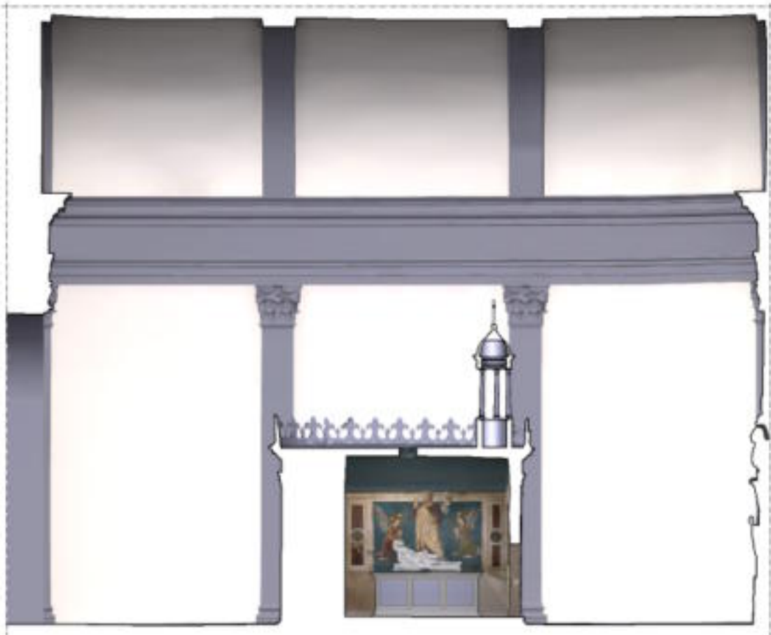
Figure 14. Long section of the Rucellai's Chapel and the Saint Sepulcher, from the 3D model (original drawing on scale 1:50).
