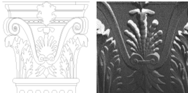
Figure 7. Photogrammetric plotting of a capital (left) and a detail of the same, scanned by laser radar (right).
