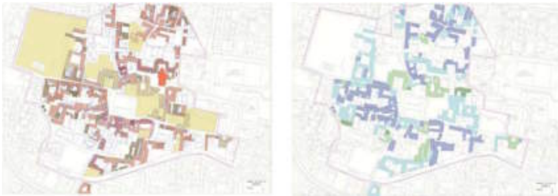
Figure 10. Inzago historic center: Identification and analysis of the architectural characteristics and Analysis of the buildings conservation problems with a preliminary preservation treatment plan. Architectural components, materials, structural characters, decay situations, transformation and alteration problems have been surveyed to underline the historical values of the buildings, in order to define urban conservation plans and guidelines.
