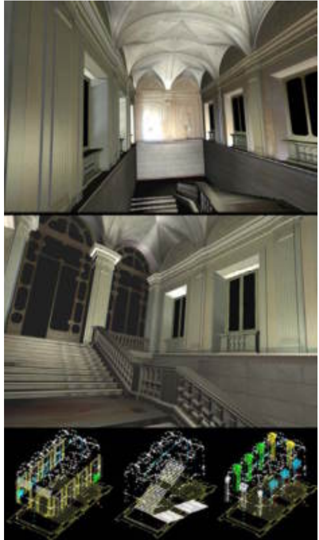
Figure 7. The model of the Scalone realized by means of the photographic sections and textured with the rectified images and the orthophoto
