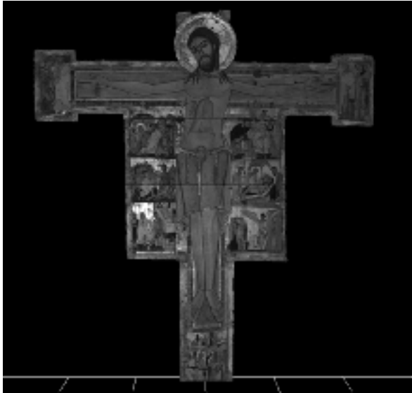
Figure 9. Laser scanner surface of Rosano cross. The scanning was made with 0.1 mm of spatial resolution
