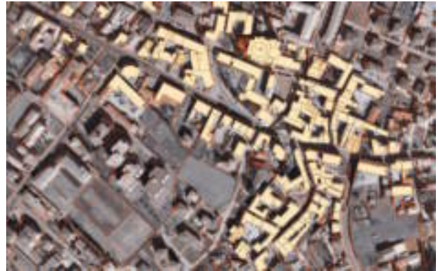
Figure 13. 3D Orthophoto of Vighizzolo. Georeferencing on CTC scale 1:2000 of buildings catalogued in DataBase (yellow colour). It was realized 3D orthophoto beginning from 3D simplified model of territory; aerial photos were realized during 1987 fly.
