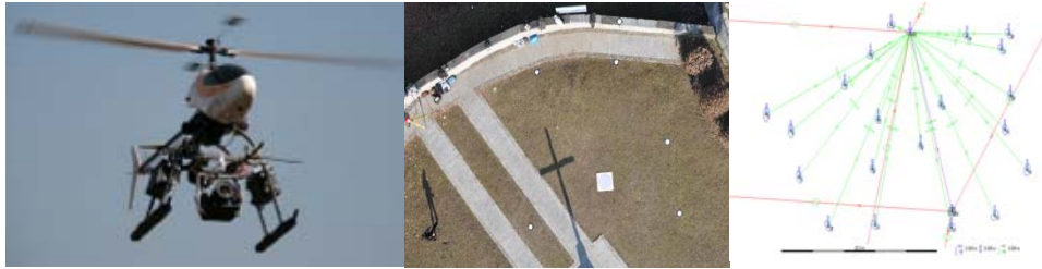
Figure 4. The UAV system, an image of the area and the scheme of theodolite/GPS measurements.
