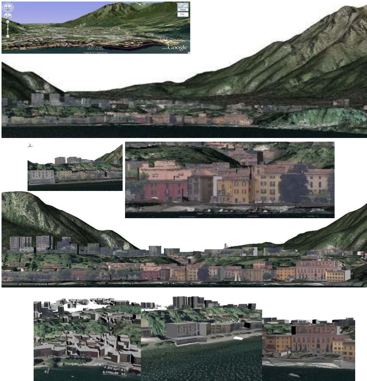
Figure. 8 (Above) Images of TopographicDB automatically textured by oriented panoramic images. (Below) VRLM model render images done within modelling sw environment (3DStudioMax)
