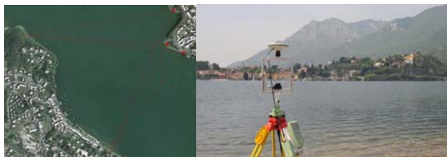
Figure 6. (Left) Test site, in red different standpoints and the lines-of-sight. (Right) ‘Photo-GPS’ system during the acquisition of images.
