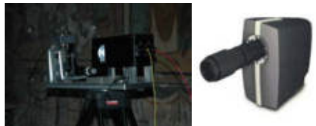
Figure 10. Laser scanner prototype Sidart 100 and multi-spectral camera used in our tests
