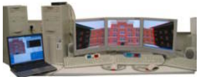
Figure 3. OpenGL-cluster containing one client and three servers
