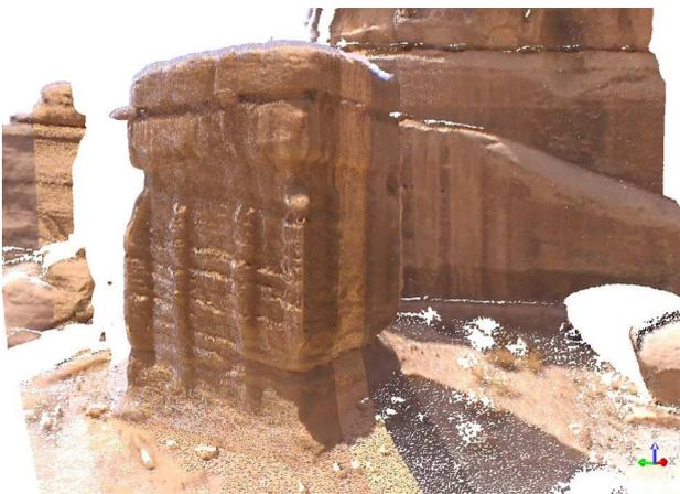
Figure 3. Point clouds coloured from the scanner, view after registration
