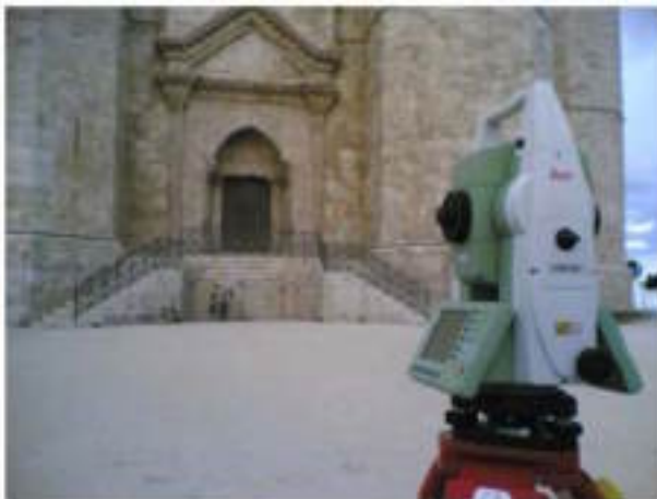
Figure 7. Total Station for the topographical surveying
