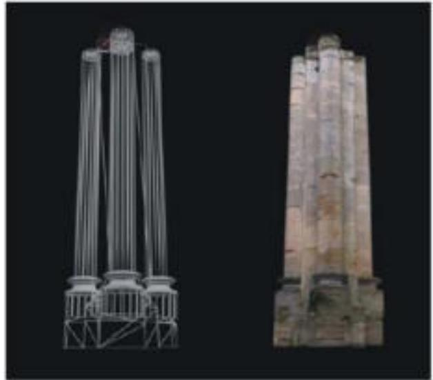
Figure 12 Wireframe and solid (with photorealistic textures) of the column of the sacristy.
