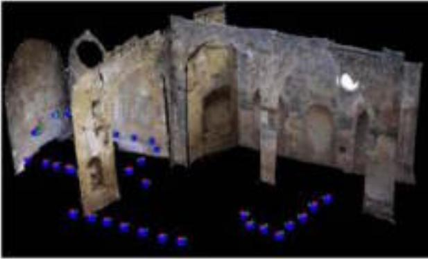
Figure 10. Partial 3D model of the church. Left chapel wall and vault textures have been suppressed to allow the visualization of the camera positions inside the chapel (screen capture from Photomodeler©).
