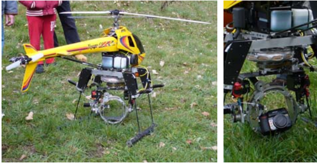
Figures 10-11 The Voyager G8 RR mini-helicopter (left), the Nikon Coolpix 8400 set up on the mechanical system (right)
