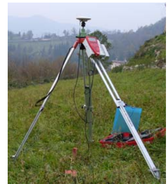
Figures 4-5 GPS network scheme (left) Leica GPS System 500 during the acquisition (right)
