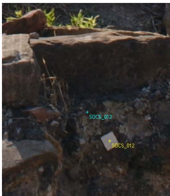
Figure 5 Misalignment between the target on the scan and on the photo
