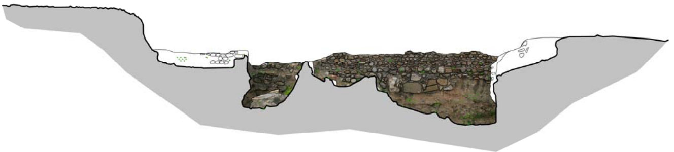
Figure 15 The orthophoto of the East wall integrated in the 2D section drawing 1:50 (not in scale)
