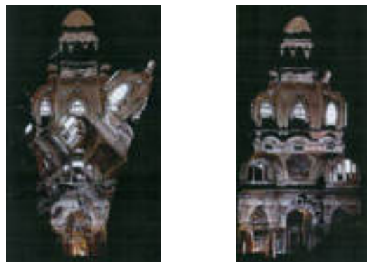
Fig. 6 – Non georeferenced point clouds on the left; georeferenced point clouds on the right.
