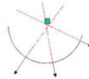
Figure 5: 2D cut of the voting geometry. Distances between lines (red) handled by the normales (black) and the voxel centers (green) are summed
