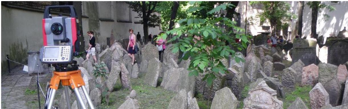
Figure 2: Measurement with reflectorless total station in exterior of Ceremonial Hall
