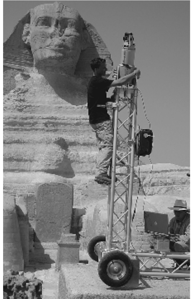
Figure 6. Mobile Scanning Platform MSP250 as used during a project in Egypt. (Photo: Wolfgang Neubauer)
