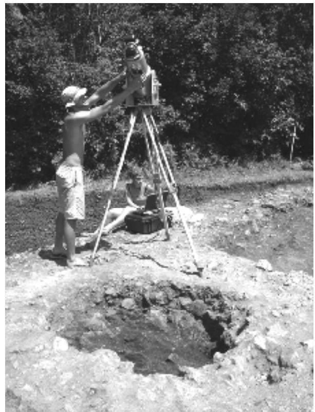
Figure 1. Schwarzenbach: Riegl LMS-Z210i 3D laser scanner with a NIKON D100 digital SLR camera mounted on top (Photo: Martin Fera).
