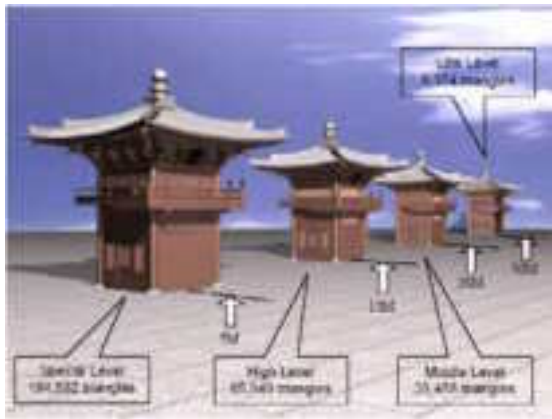
Figure 3. Bell Tower's models of different LODs
