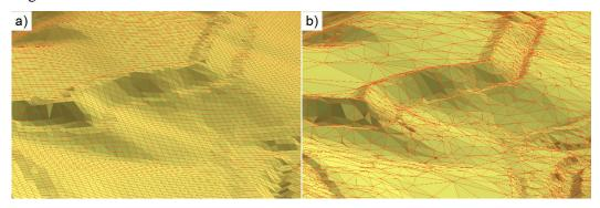
**Figure 3:** Visualization of DTM (source: archive of Land Survey Office). Left: visualization of grid DTM, right: visualization of TIN DTM
