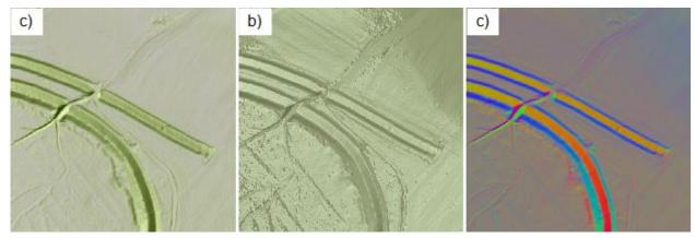
**Figure 5:** Alternative visualizations of elevation data: a) shaded relief with transparency slope layer, b) shaded relief with transparency aspect layer, c) color composed RGB shaded relief.
