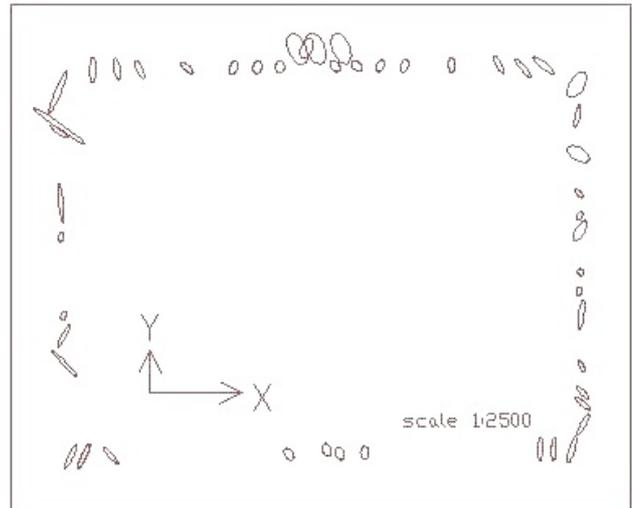
Figure 3. Error ellipses of the control points on the wall
