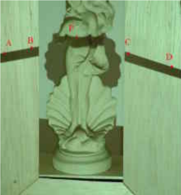
Figure 2. A photograph of the object, the control device and the projected raster lines upon them
