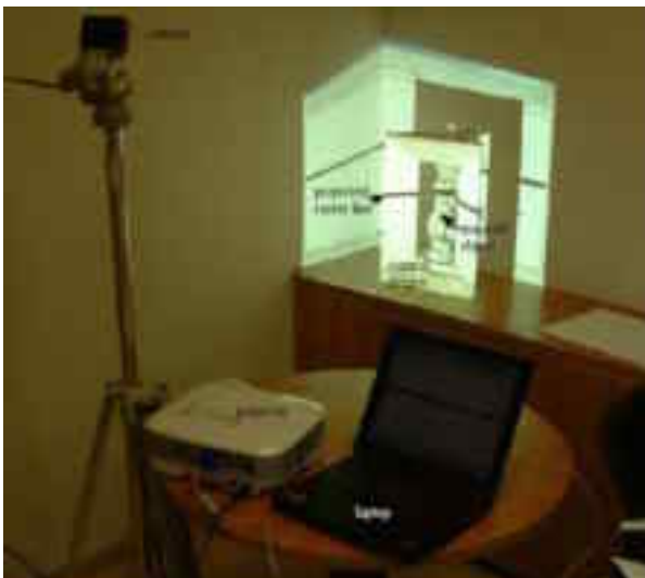
Figure 1. The rasterstereographic set up consisting of the object under test, a control device, a projector and a camera
