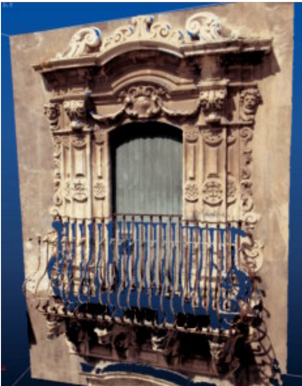
Figure 14. Projection of the photographic image on the mesh
