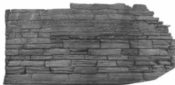
Figure 4: Mosaic of several orthoimages produced from coloured DSM points of a cylindrical tower.
