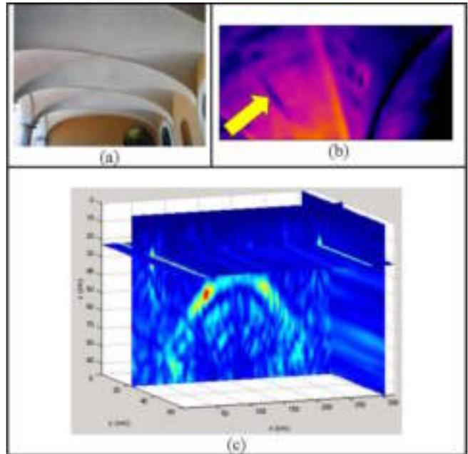
Figure 3. Photograph of the depressed multi-centred profile porch vaults (a). Detection of inclined tie rod hidden by the plaster of the vault by active thermography (yellow arrow - b). 3D GPR volume measured with a 1GHz antenna above one of the porch vault (c).
