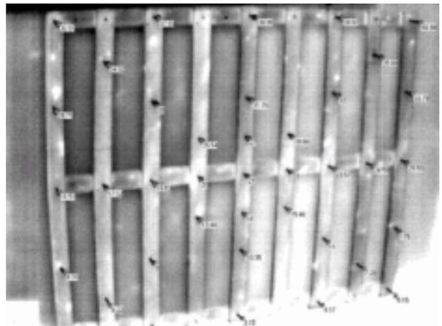
Figure 7. Thermal image of the calibration polygon with superimposed positions of GCPs
