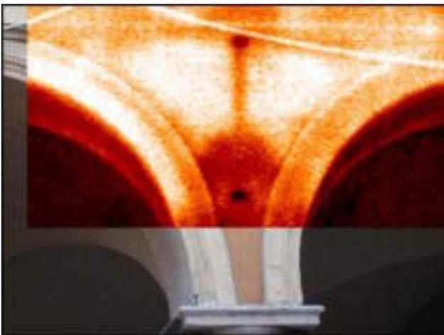
Figure 2. Thermographic inspection of the external porch overlaid to a photograph.
