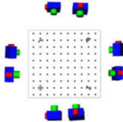
Figure 3. The calibration test-field and the images acquisition position.
