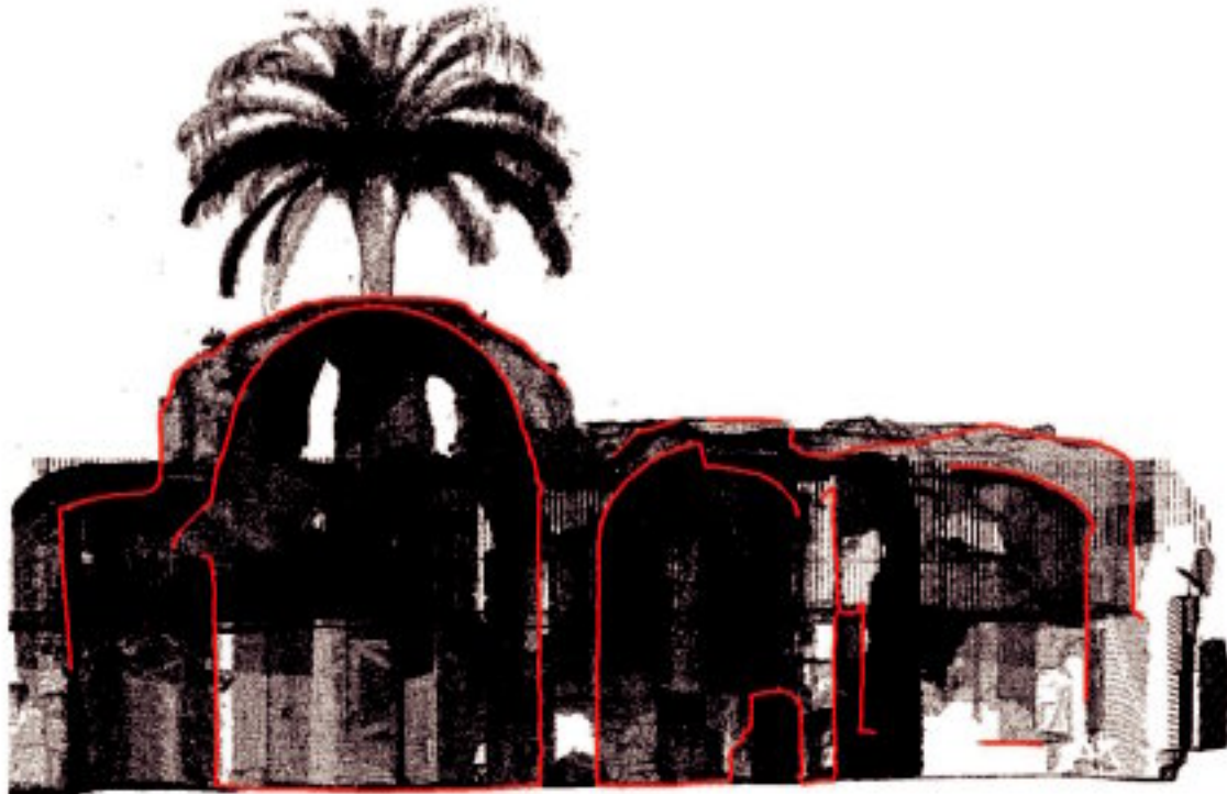
Figure 8. Vertical section along the plane passing through one of the octagonal plan's diagonals
