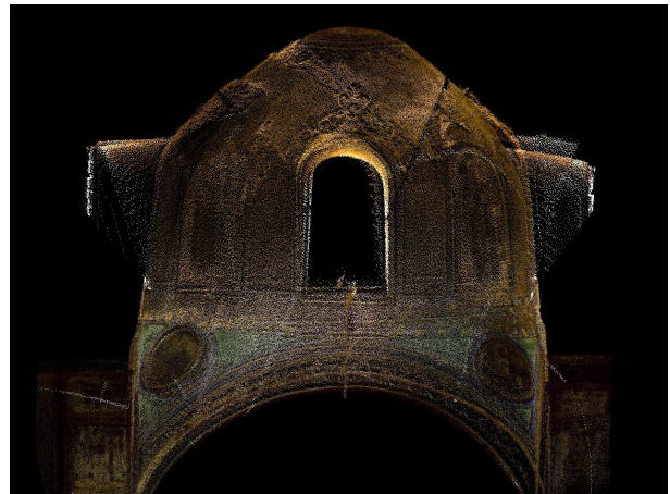
Figure 3. Different views obtained from point cloud of inner facades of Sille Ayai Eleni Church
