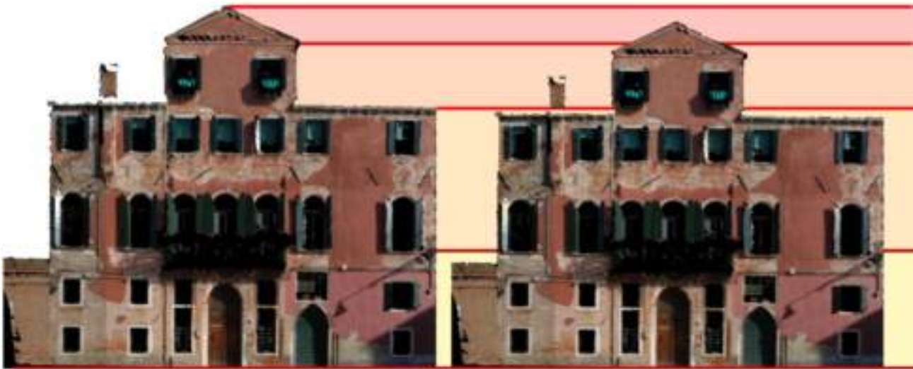
Figure 5. Growing error in orthophoto due to errors in vertical axis definition
