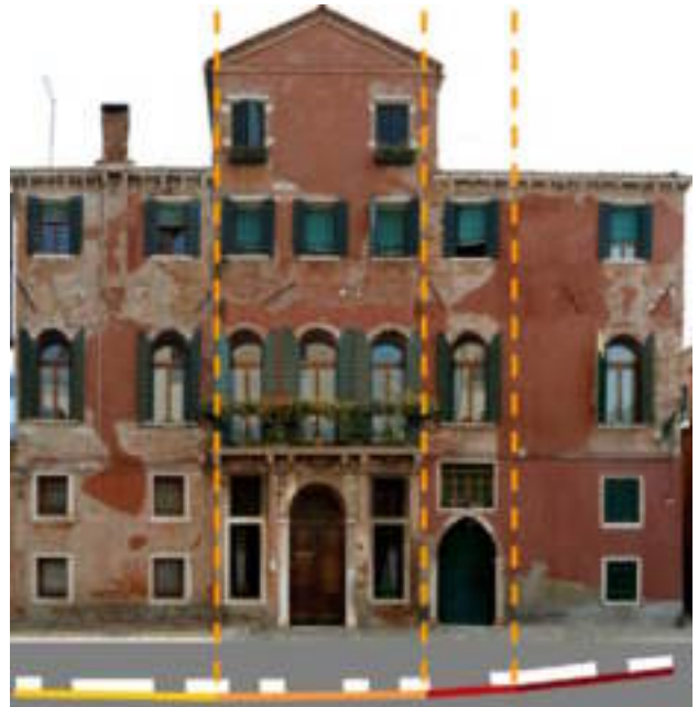
Figure 8. Rectification and development respect different planes
