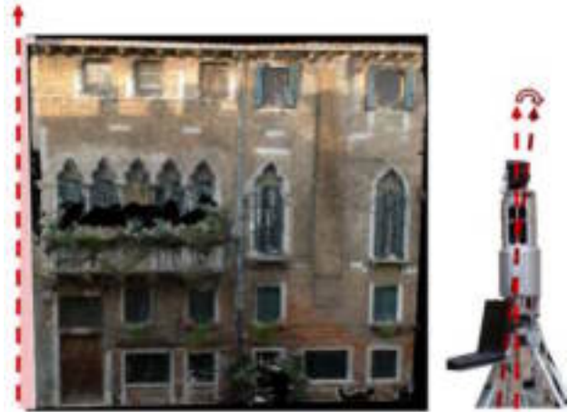
Figure 3. Instrumental verticality is fundamental in a façade control survey to avoid errors in profiles extraction
