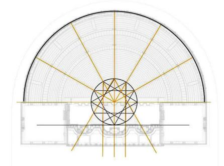
Figure 3: The theory of Vitruvius: frame of the animation reproducing the construction of an ideal theatre generated by an equilateral triangle.
