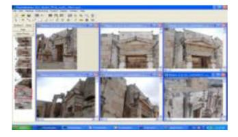
Figure 4. Several photos from different angles with known focal length, using control points for the Scine of the Southern theatre
