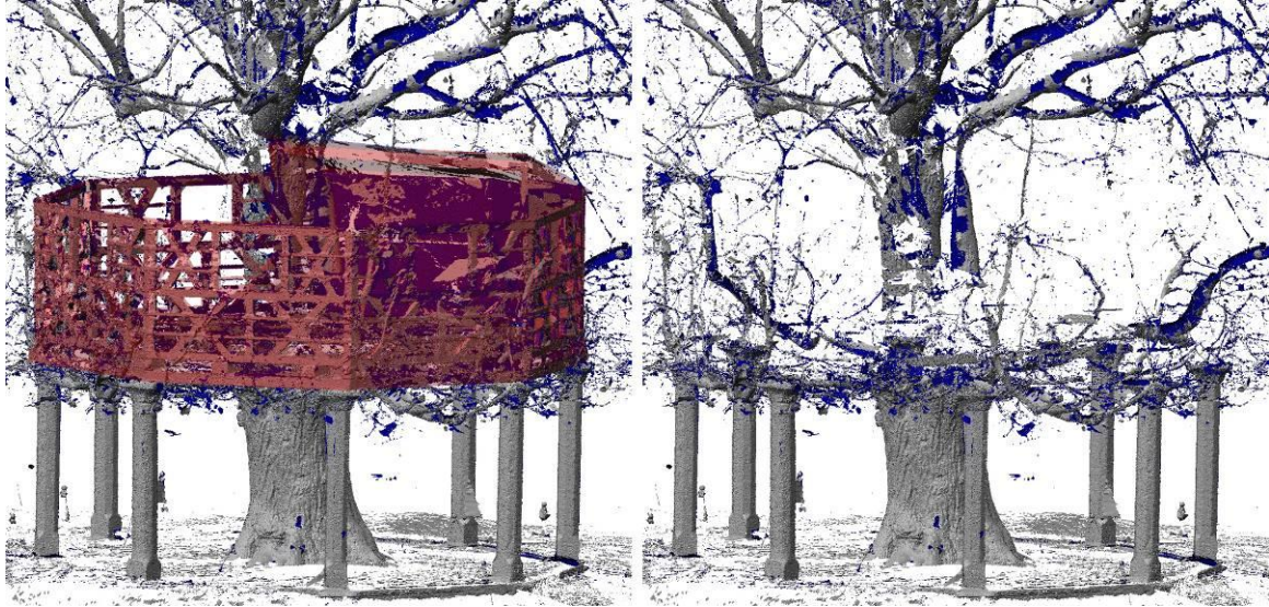
Figure 3: Segmentation of the point cloud using the photogrammetrically achieved surface model (red)
