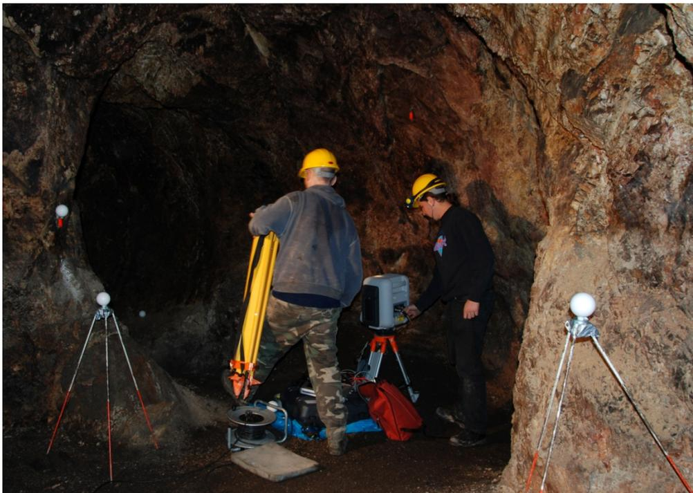
Fig.1: laser scanning down in a prehistoric mining site
