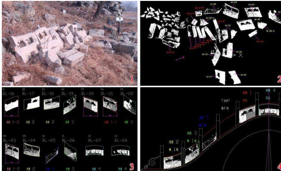
Figure 3: 3D Laser Scan and virtual reassemble of the Bilan-Bridge (1. 3D Laser Scan at the sites; 2. Primitive spatial models; 3. Processed models of the bridge railing; 4. bridge railings were virtual reassembled in infallible location)
