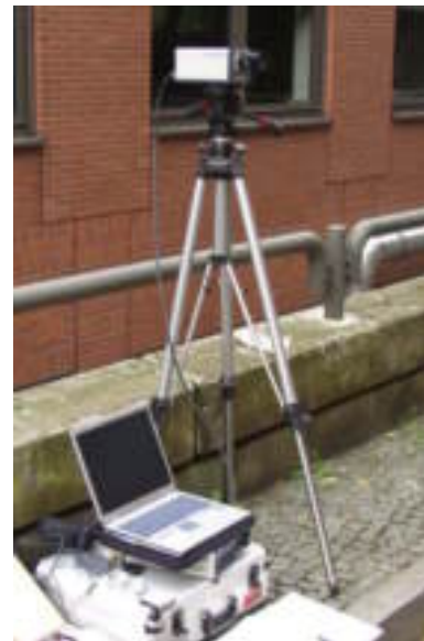
Figure 3. IR-Vidicon-camera with controller and notebook
