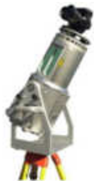
Figure 8. Laserscanner Riegl LMS-Z420i [Riegl, 2004]
