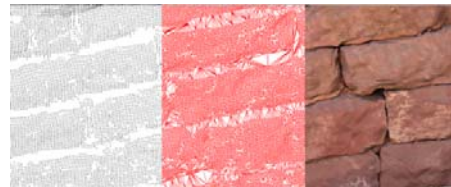
Fig. 11. (a) point cloud (b) wireframe (c) textured model of a wall
