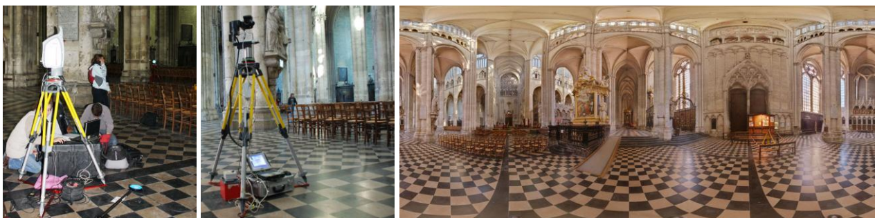
Figure 5: Laser scanner and Rodeon station on the same point + resulting panoramic image
