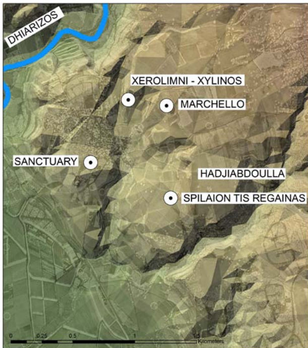
Figure 6. 3-D reconstruction of the terrain using orthophotos and TIN
