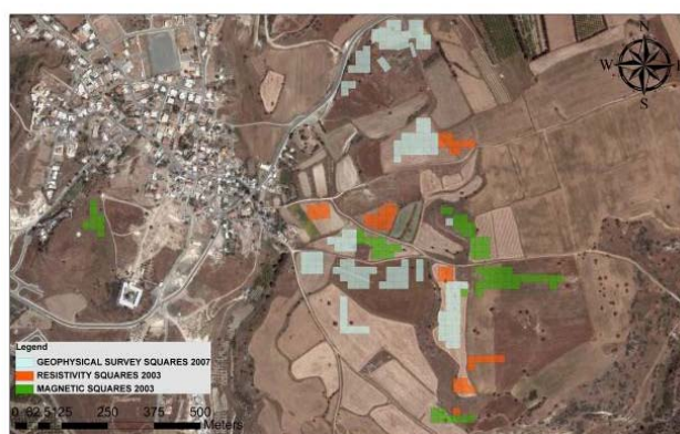
Figure 3. Outline of the geophysical grids that were explored during the 2003 and 2007 field season. A high degree of overlap existed among the different methodologies in order to enhance the interpretation of the data.
