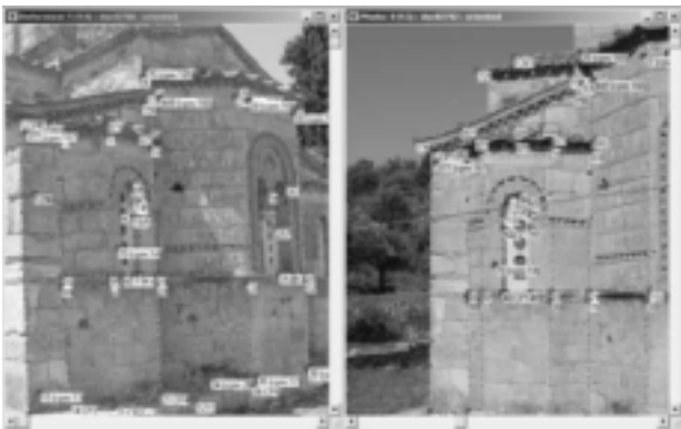
Figure 3. Location and measurement of homologue points in PhotoModeler
