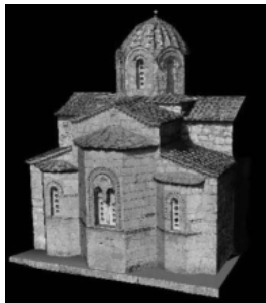
Figure 5. 3D textured model produced from the PhotoModeler using the digital images
