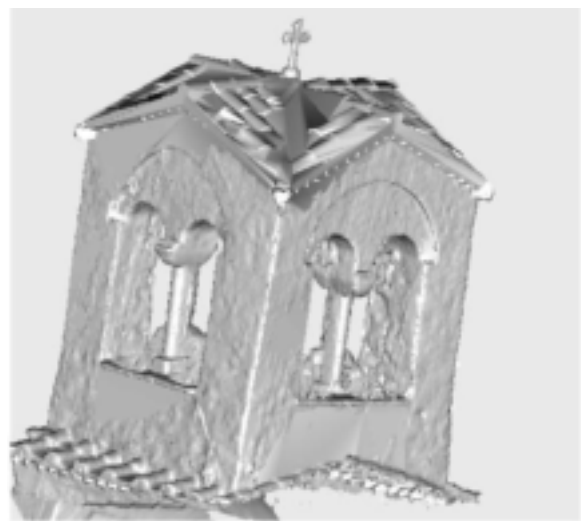
Figure 8. Hybrid geometric model of the bell tower
