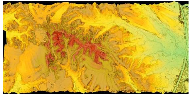
Figure 3. DTM Gradation map by airborne laser data
