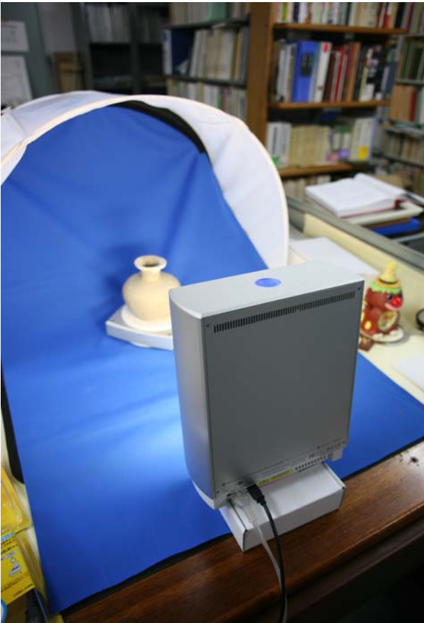
Figure1. Laser Scanning by the Low-cost scanner.
