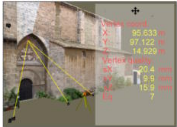
Figure 10. Another example for the visualization of quality: the activated vertex was determined by a spatial intersection of three photogrammetric observation rays and one virtual shape ( 3*2+1=7 )
