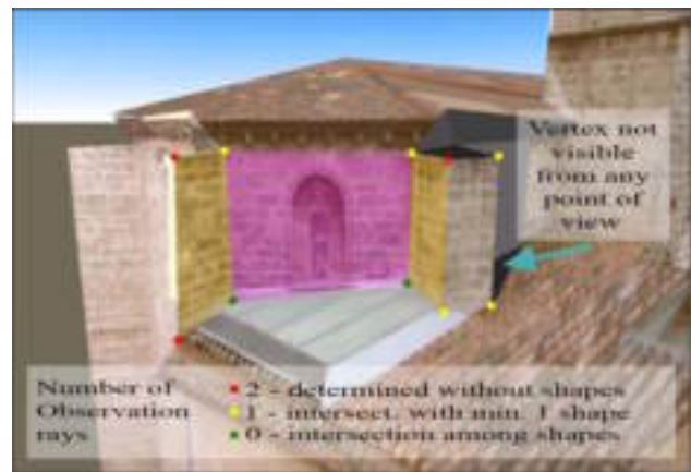
Figure 5: Various model vertices could only be observed from one point of view, which impeded the spatial intersection of these points. But using virtual shapes, they could still be determined as intersections of observation rays with shapes.
