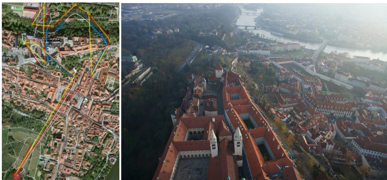
Figure 5: Flight trajectory and shooting position plan and an example of realized photography
