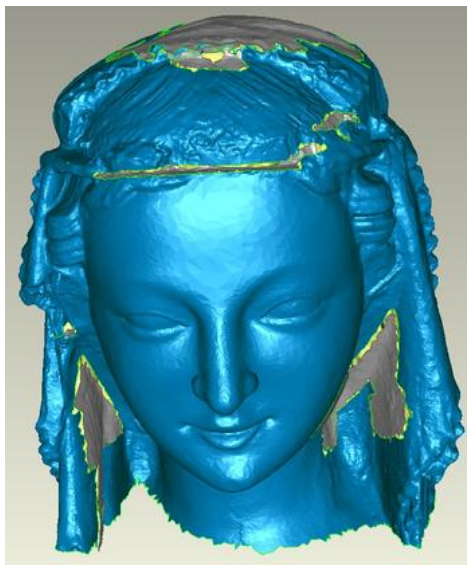
Figure 5: Surfaces filled in from the CT data (grey) to the LORS data (blue) in unreachable areas for LORS The final model is presented on the Figure 1 and a detail on the Figure 6.
