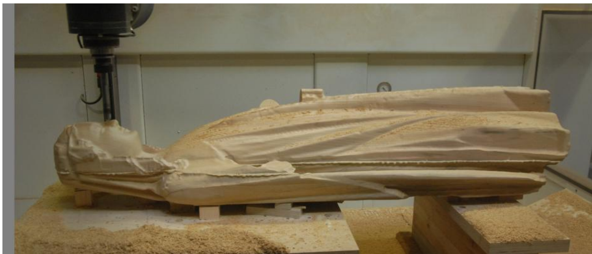
Figure 10: 3D milling cutting – CNC
