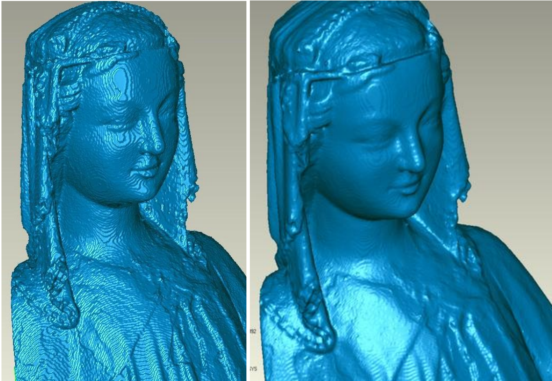
Figure 3: Model exported from the DeVIDE software and model after post processing in Geomagic Studio
