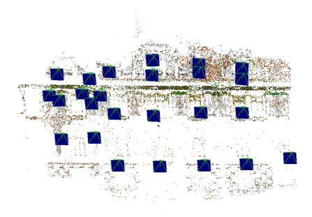
Figure 5: Reconstructed projection centers
