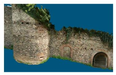
**Figure 6:** 3D meshed and textured model obtained on the lower part of the compound wall, covered with vegetation
