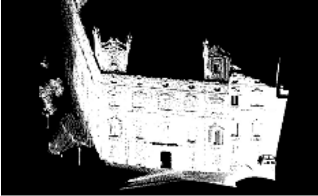
Fig. 2. 3D Point cloud after registration.
