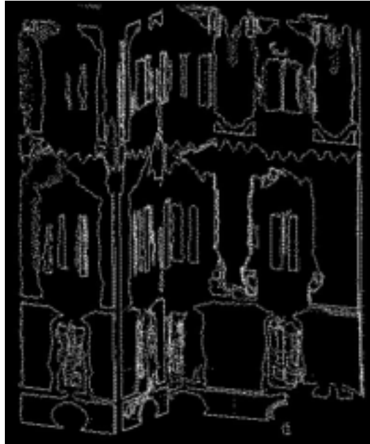
Fig. 9. View of bounds extracted with a resolution of 50 mm.
