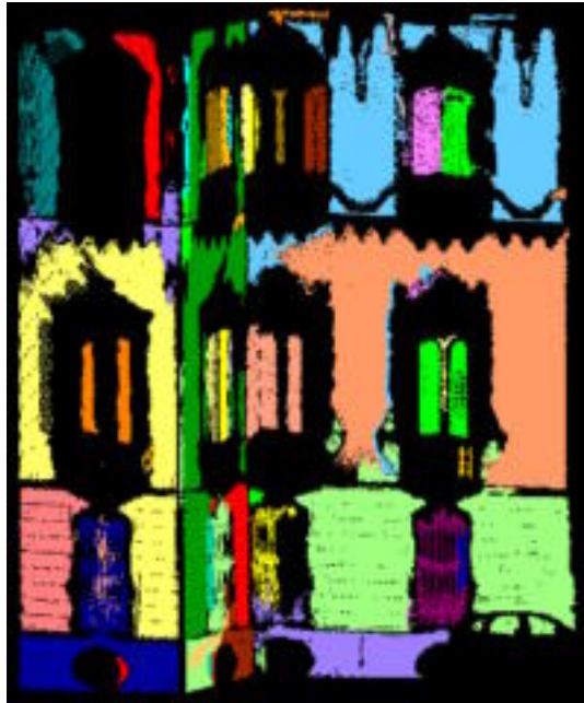
Fig. 7. View of the result of the segmentation process. Each plane is represented in a different colour.
