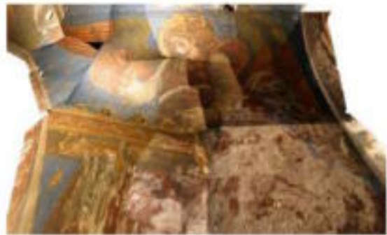
Figure 5. Example of rough mosaic. Original input image colours (without correction) and inappropriate local geometric corrections
