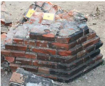
**Figure 5:** Numbering of fallen brick pieces prior to laser scanning
