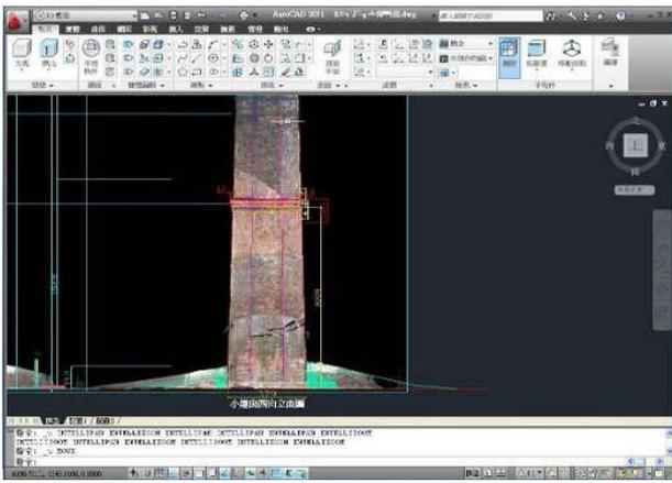
**Figure 8:** Using the 3D point cloud section data of south chimney to generate the 3D model
