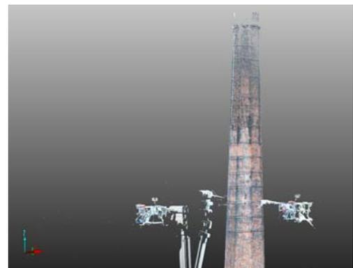
Figure 11: Rapid digitalisation scanning technique was used to obtain the 3D surrounding site view
