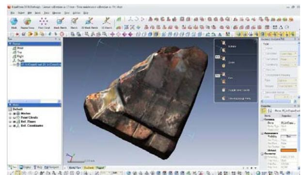
Figure 14: The construction and coloration process of a piece of ruin brick using MESH
