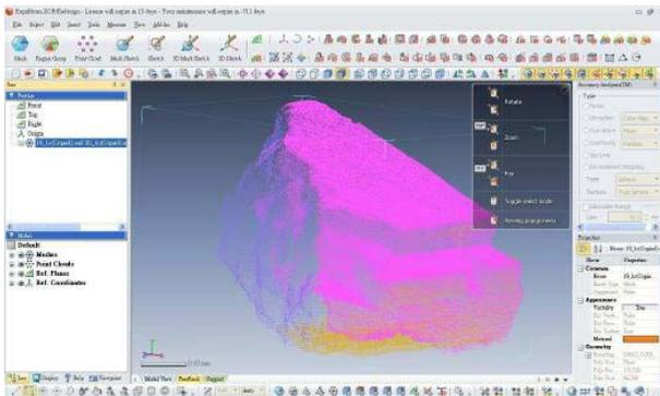
Figure 12: Point cloud data obtained from various positions are represented by different colour tones
