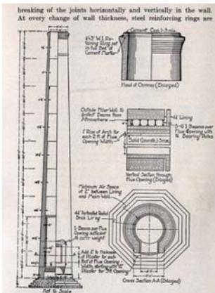
**Figure 2:** The chimney of Same-tō brick factory was made a traditional western-style method[1]
