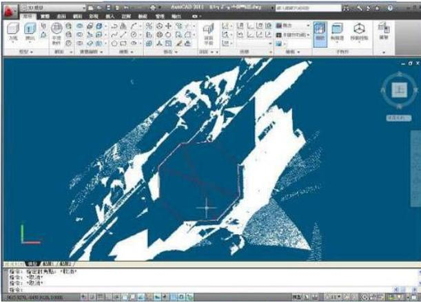
**Figure 7:** 3D point cloud data of south chimney foundation subjected to in-plane orthographic projection
